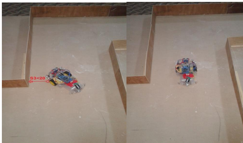
Figure (12): The robot approaching the wall from the left side, and when it changed the direction of its movement.
