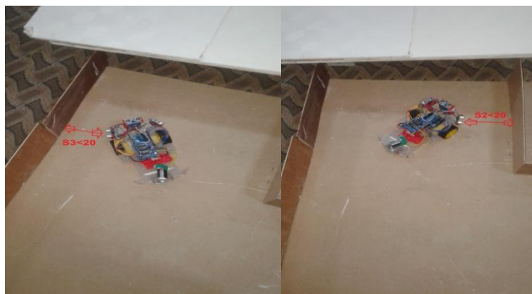
Figure (14): The robot approaching the wall from the left side and then from the right side.
