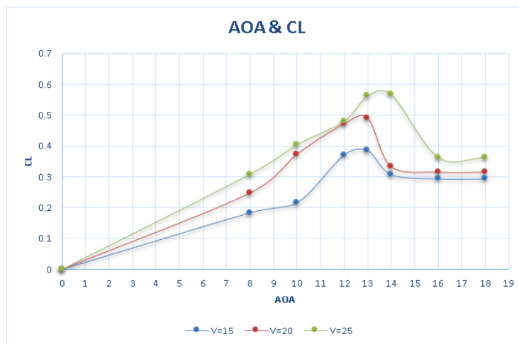
Figure 3: Experimental Comparison of Angle of Attack (AOA) and Lift Coefficient ( C_L ).
