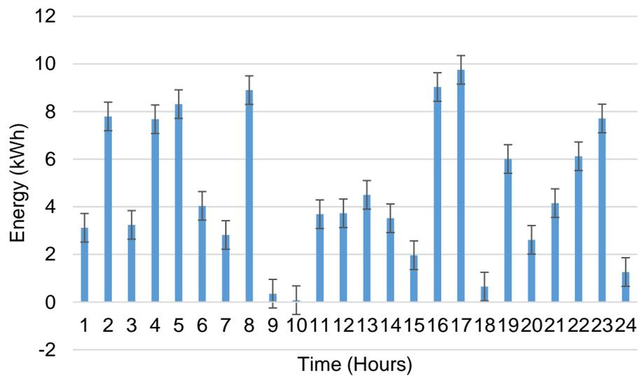
Figure 3. PV output energy produced to charge electric vehicle.
