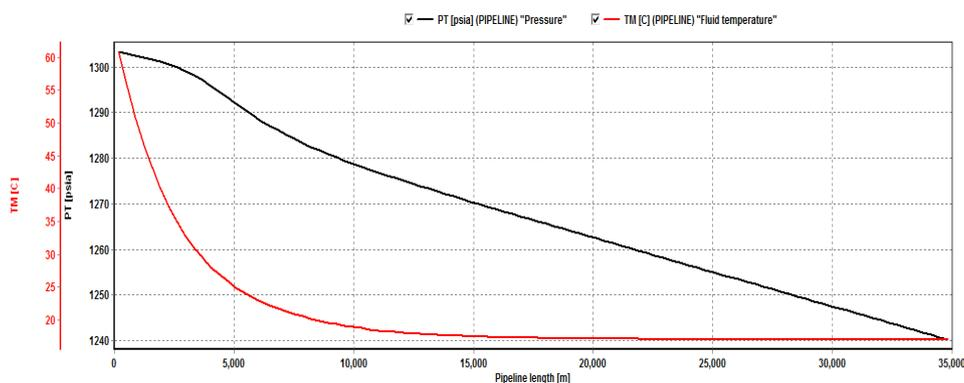
**Figure 7.** Temperature and pressure profiles of the crude oil along the pipeline (Option 2-TCP)
