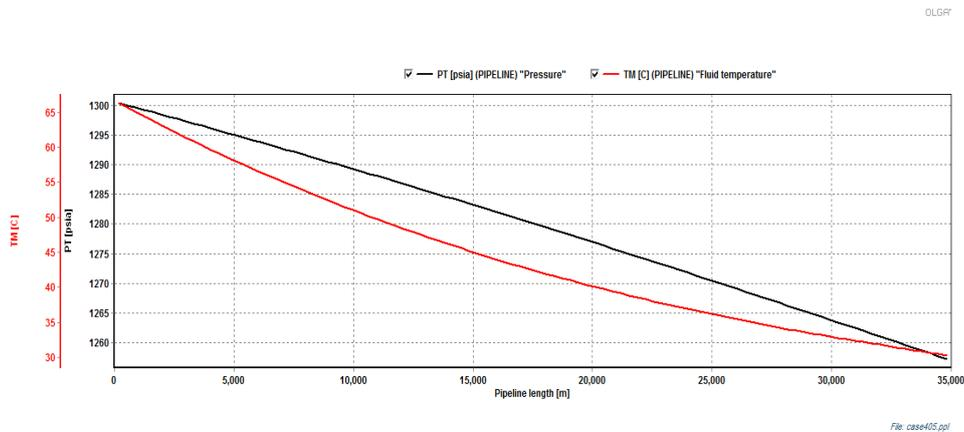
**Figure 12.** Temperature and pressure Profiles of the crude oil along the pipeline (Option 3-Insulated TCP).
