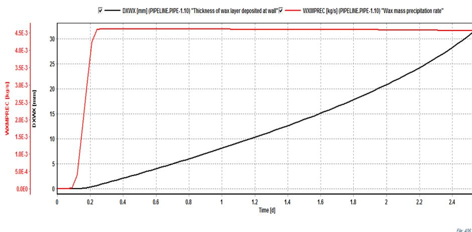
**Figure 20.** Wax deposition trend of Option 1 CS (The front section of the pipeline)
