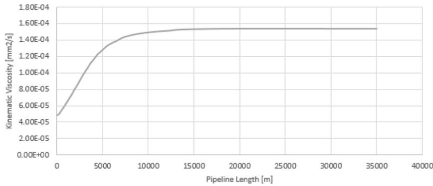
**Figure 11.** Profile of Kinematic viscosity profile of the crude oil along the pipeline (Option 2- TCP).
