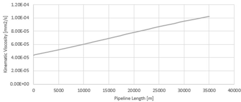
**Figure 16.** Profile of Kinematic viscosity profile of the crude oil along the pipeline (Option 3- Insulated TCP)
