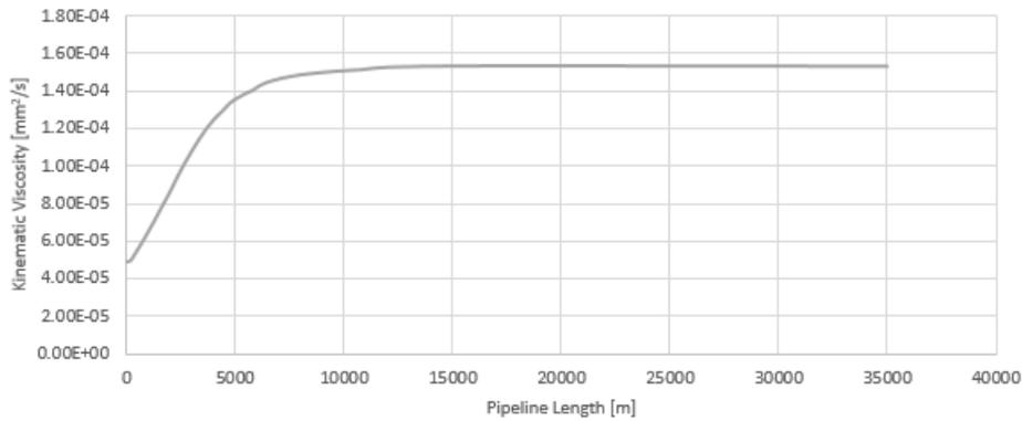
**Figure 6.** Profile of Kinematic viscosity profile of the crude oil along the pipeline (Option 1- CS)
