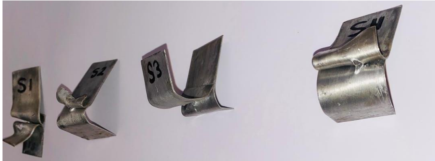
Figure (7): Fractured samples after peel test.
