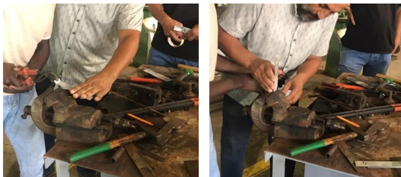
Figure (6): The peel test.
