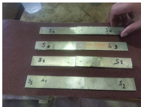
Figure (3): Real welded samples.
