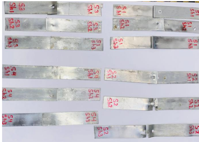
Figure (8): Fractured samples after tension–shear tests.
