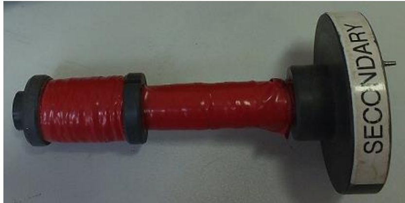
Figure 10b. Sample holder and pick-up coil.
