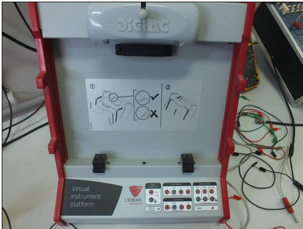
Figure 7a. DIGIAC 3000 Platform device (signal generator)
