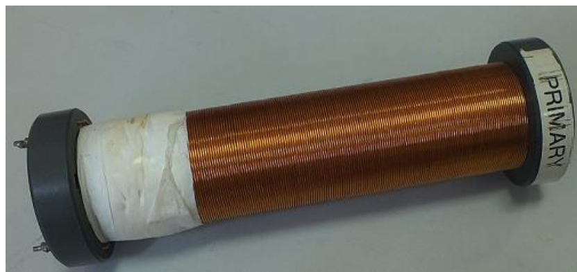
Figure 10 a. Excitation coil (Primary coil)
