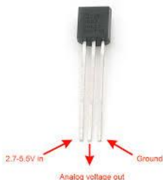
Figure 12 b. The temperature sensor LM35
