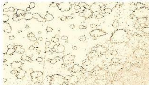
Figure. (4-c): Cooled in water with detection of carbides.
